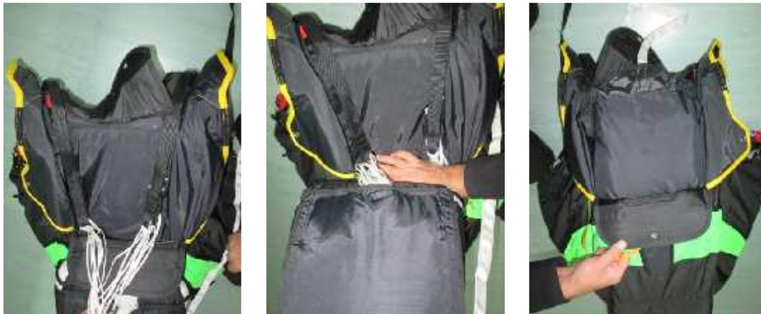
Fold the Rescue Static Line (RSL) on to the free bag.
