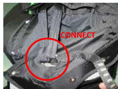
Insert the rescue in the container under the seat, with the lines face down.
