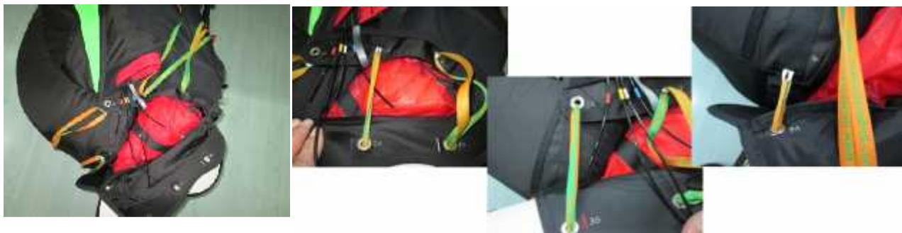
Pull the cord trough the grommets and pin all the loops with the handles closing cable from 1 to 4. For your convenience there are different color markers on each cable and each grommet.
