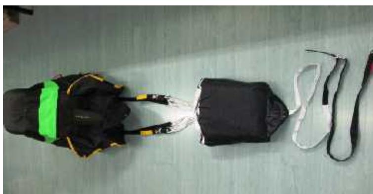
Now turn the free bag and put it in to the harness container with the line pocket down.
