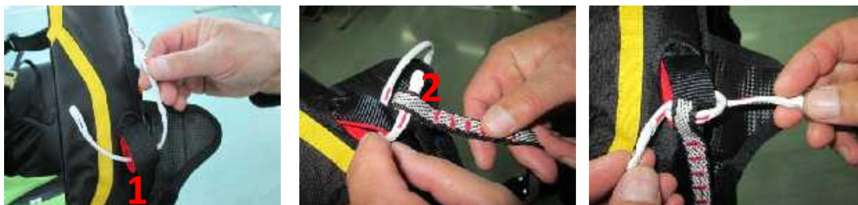
Insert the soft link line in the red attachment point (1) located at each shoulder belt ( under the magnets ), and the rescue attachment line (2).
