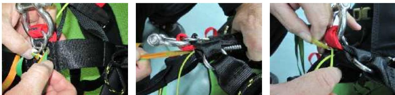
The Loop must be on the back side of the grommet. Lock with the cutaway cable and insert the cable end into the belt pocket
